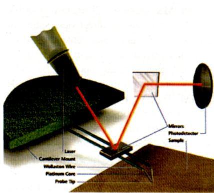
Fig. 1: Schematic of probe set-up
