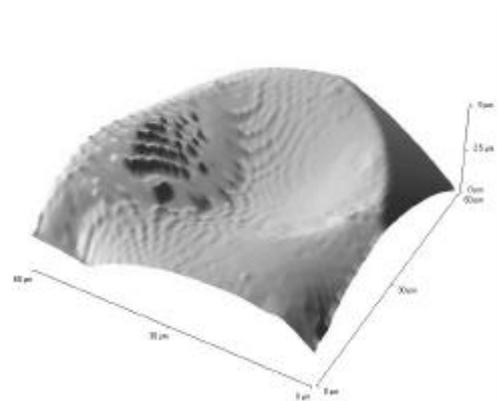
Figure 2. Pyrolysis crater (50 $\mu$ m across, 5  $\mu$ m deep) in a 100  $\mu$ m diameter polystyrene bead.
