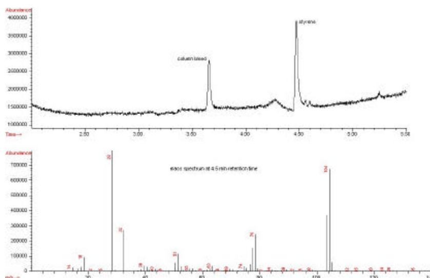
Figure 3. GC-MS analysis of evolved gases from the ablated area in figure 2 showing styrene monomer generated by pyrolysis of the polymer.
