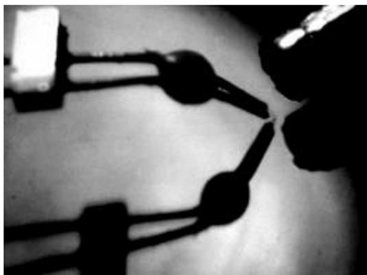
Figure 1. Thermal SPM probe (left) and end of sorbent tube.
