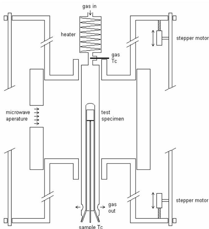
**Figure 4.** TM010 cavity and sample holder design (schematic).
