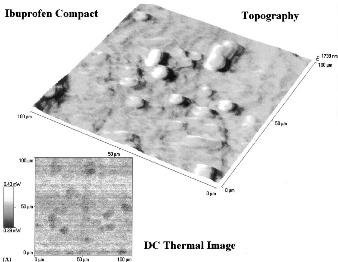
Fig. 1. Micro-thermal analysis images of (a) ibuprofen and (b) HPMC alone, showing topography and thermal conductivity.
