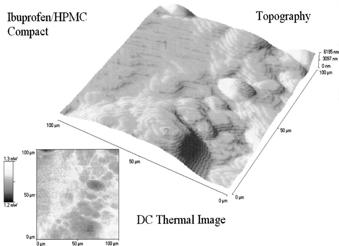
Fig. 3. Topographic and thermal conductivity image of ibuprofen-HPMC compacts.
