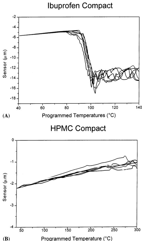
Fig. 2. Localised thermal analysis for compacts of (a) ibuprofen and (b) HPMC.
