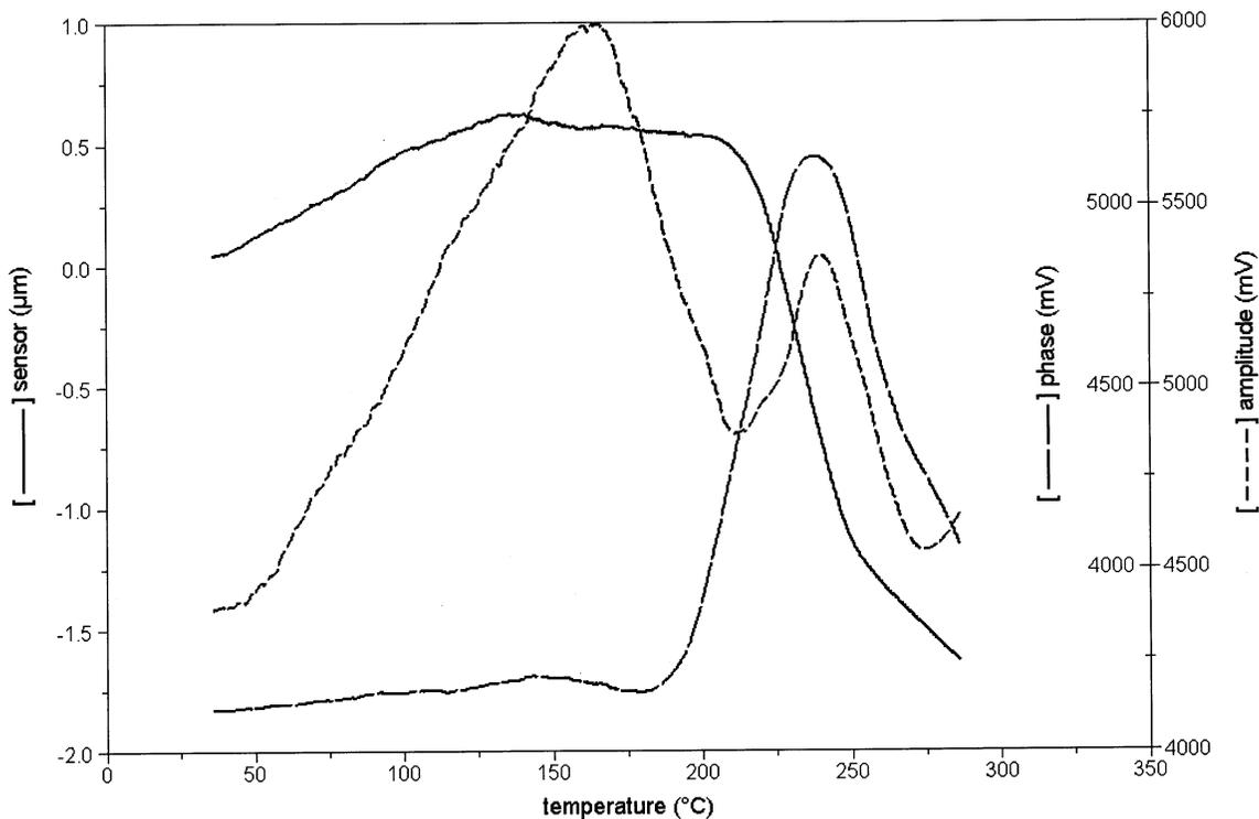
Fig. 9. Localised DMA of nylon showing the glass transition at 140°C and melting at 230°C.
