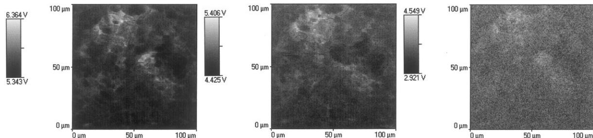
Fig. 4. AC thermal images of the voltage required to modulate the probe temperature with an amplitude of 5°C at 10 kHz (left), 30 kHz (middle) and 100 kHz (right).
