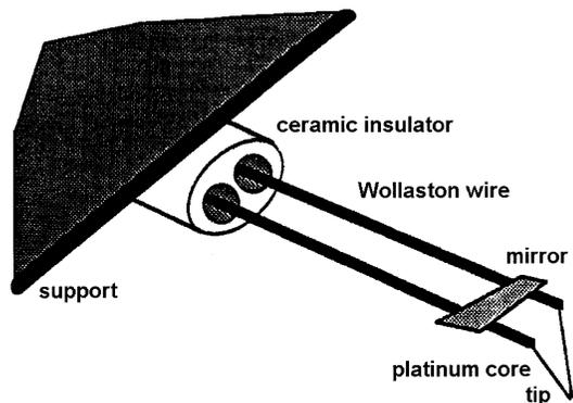
Fig. 2. Thermal probe (schematic).
