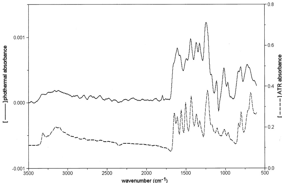
Fig. 12. Photothermal absorption spectrum of paracetamol (solid line) acquired using the thermal probe—the conventional ATR spectrum is shown (broken line) for comparison.
