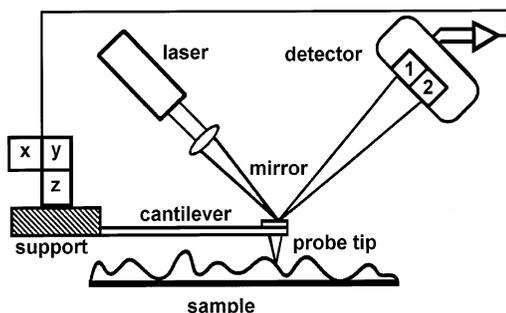
Fig. 1. Atomic force microscope (schematic).
