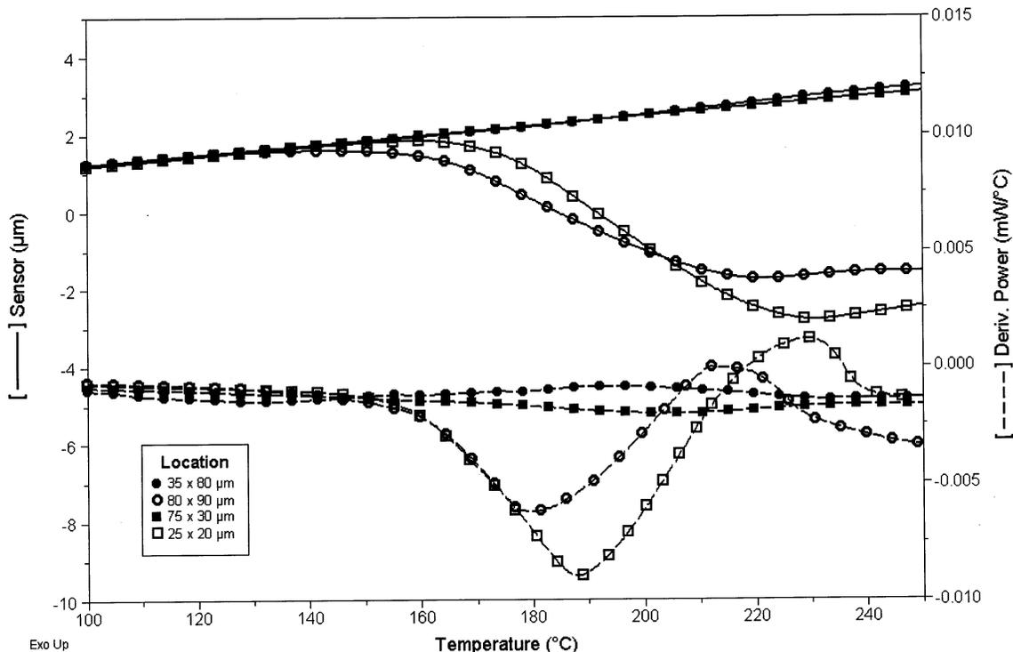
Fig. 8. Localised TMA (solid line) and DTA (broken line) curves for four different points on the images shown in Figs. 3–5.
