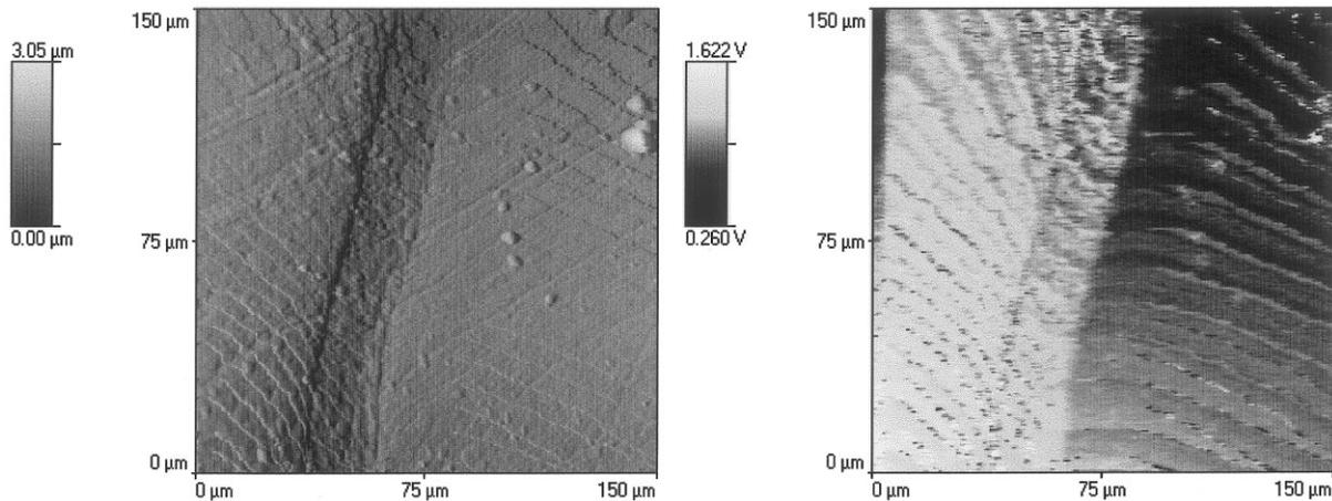
Fig. 10. Topographic (left) and thermal expansion (right) images of a polymer/metal interface. The polymer exhibits a higher thermal expansivity than the metal and shows up bright in thermal expansion image.
