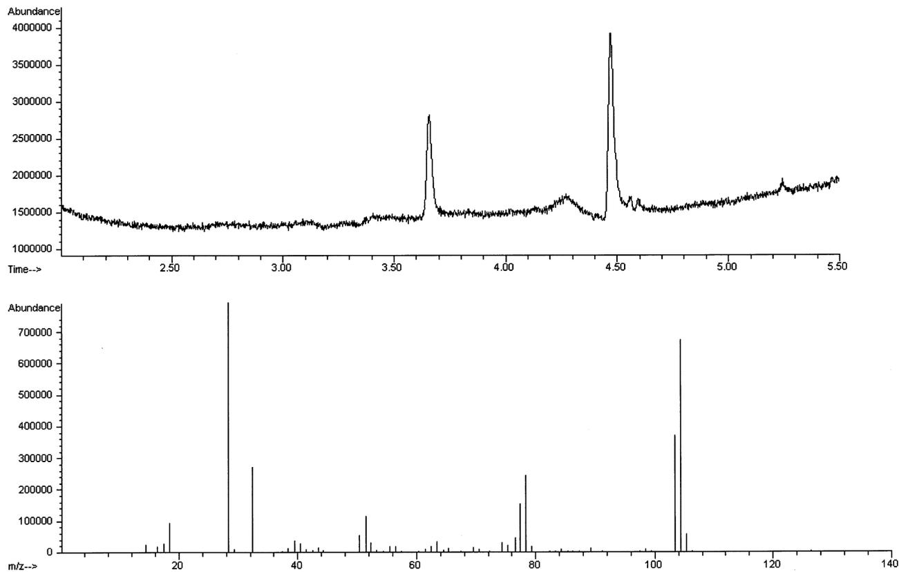
Fig. 11. Total ion chromatogram (top) from the pyrolysis of polystyrene. The peak at retention time 3.66 min is due to bleed from the GC column. The peak at 4.47 min is identified as styrene monomer (mass spectrum shown beneath) arising from the thermal degradation of the polymer.
