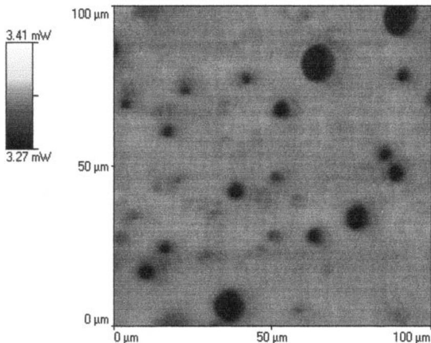
**FIGURE 2.** Thermal conductivity contrast image of a polymer blend. The dispersed phase has lower thermal conductivity than the matrix.
