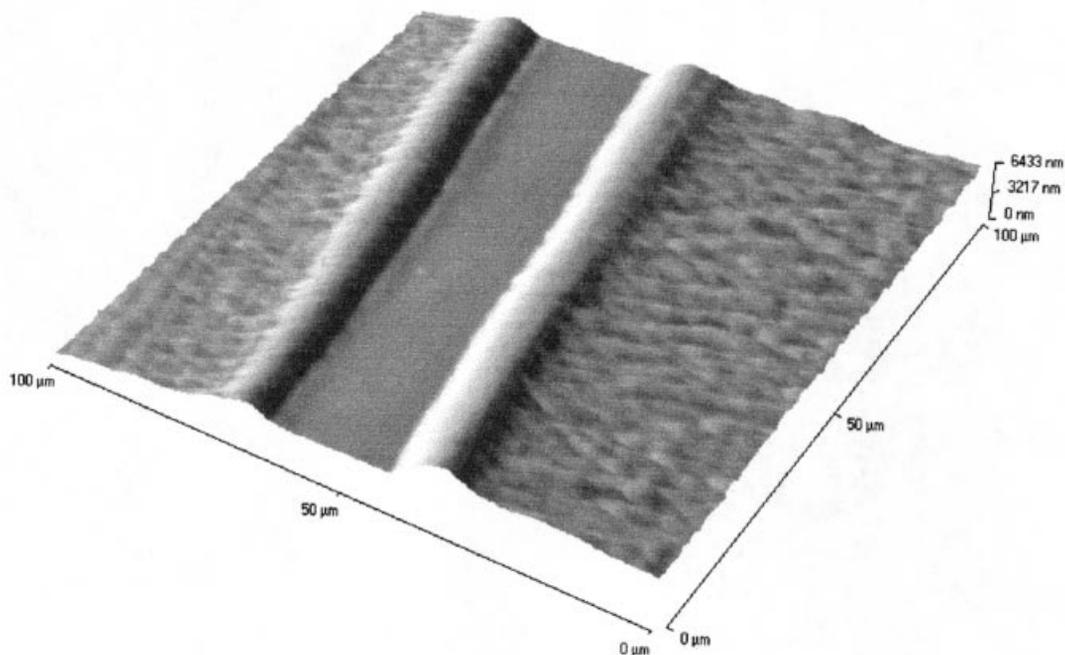
**FIGURE 3.** Three dimensional perspective topographic image of a cross-section through packaging film showing a central gas-barrier layer flanked by tie layers within the bulk film.
