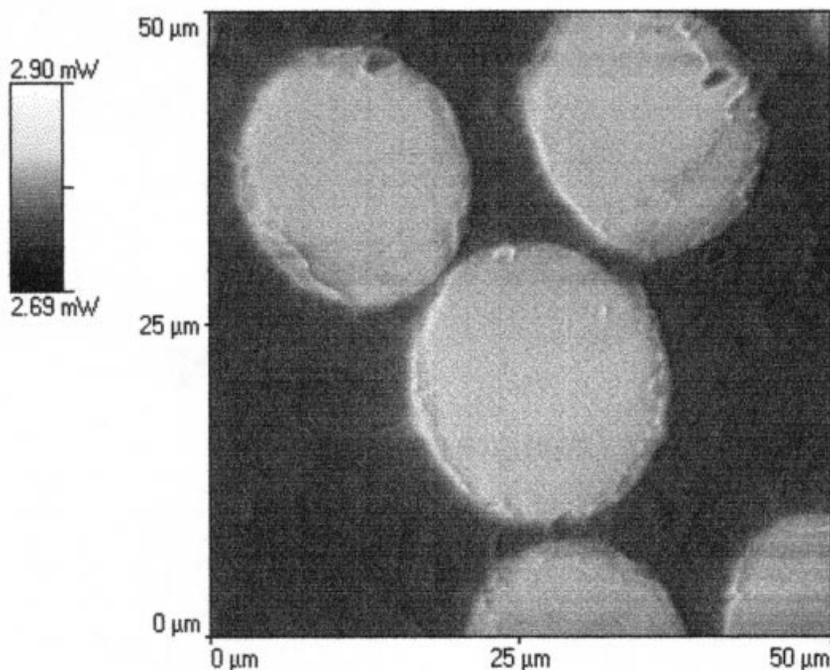
**FIGURE 1.** Thermal conductivity contrast image of glass fibres in a polymer matrix. The glass fibres are the bright (high thermal conductivity) circles.
