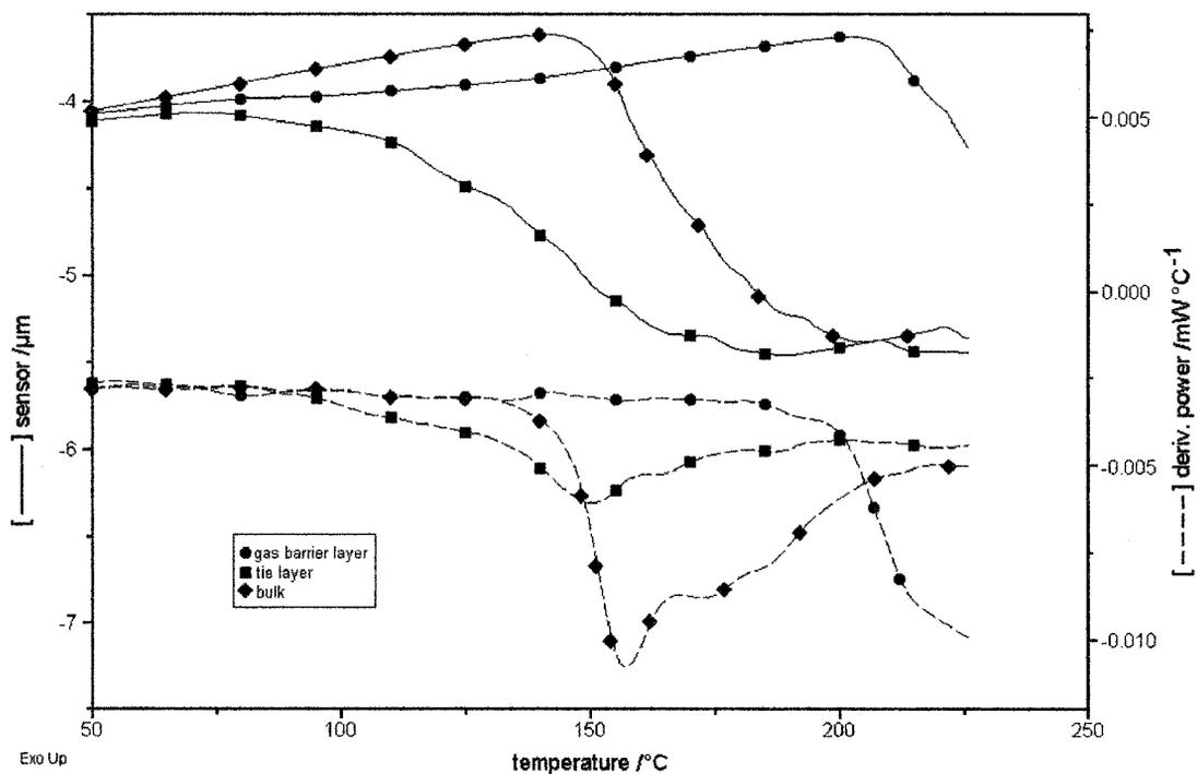
**FIGURE 4.** Localized thermal analysis of the gas barrier region, tie layer and bulk film.
