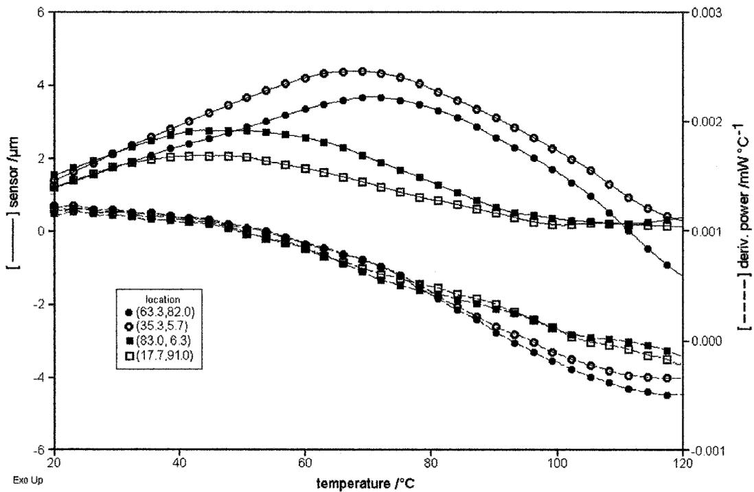
FIGURE 6. Localized thermal analysis of the blend shown in Figure 2 identifying each phase from its glass-transition (softening) temperature.
