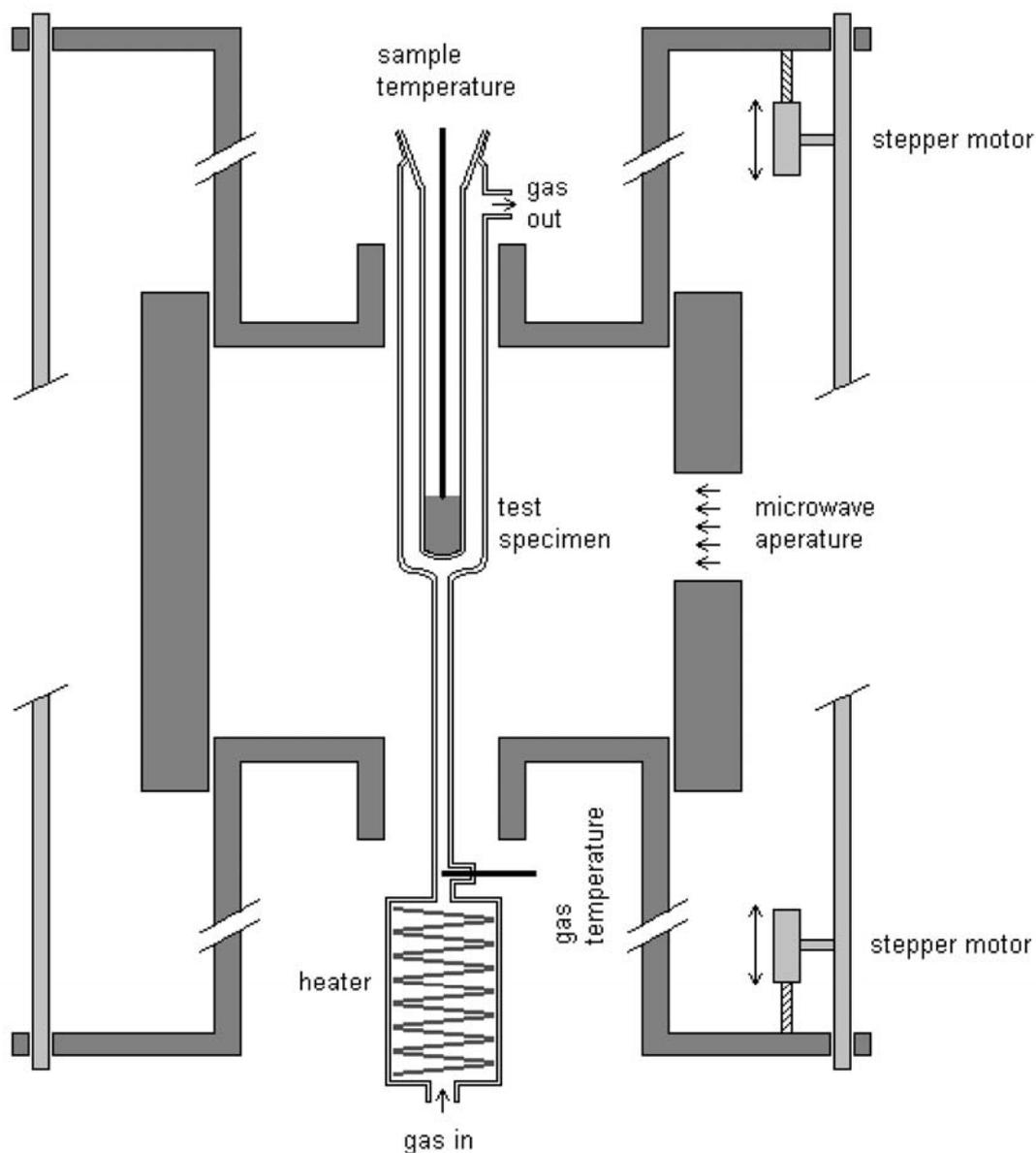
Figure 1. Schematic diagram of test cavity showing arrangement for heating sample and positions of temperature sensors.
