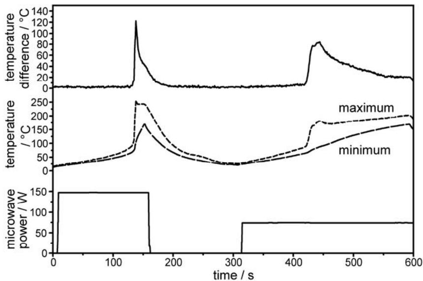
Figure 6. Temperature vs time profiles of silver iodide heated by 150 and 75 W microwave power.
