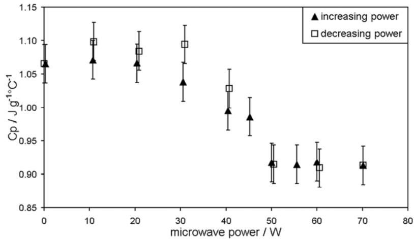
Figure 5. AC calorimetry data for silver iodide at 130°C under different levels of microwave power.
