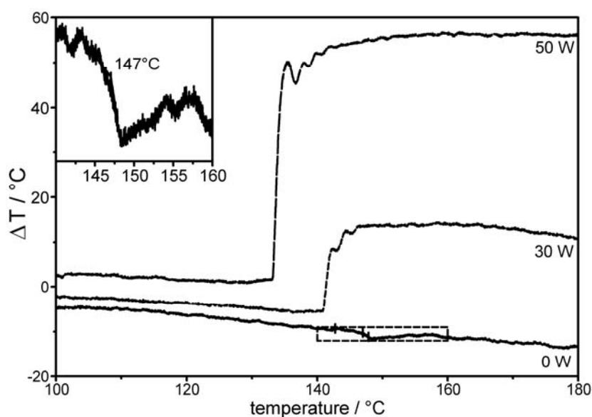
Figure 2. DTA data for silver iodide heated at  $1^{\circ}\text{C min}^{-1}$  under increasing levels of microwave power (inset shows expansion of 0 W curve in transition region).
