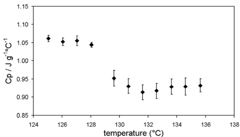
Figure 4. AC calorimetry data for silver iodide with a 50 W microwave power background.
