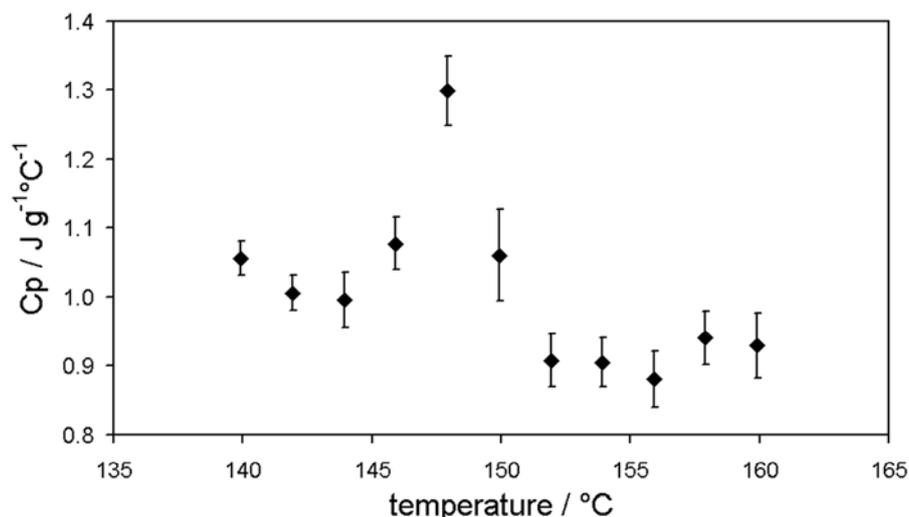
Figure 3. Heat capacity of silver iodide measured by AC calorimetry.
