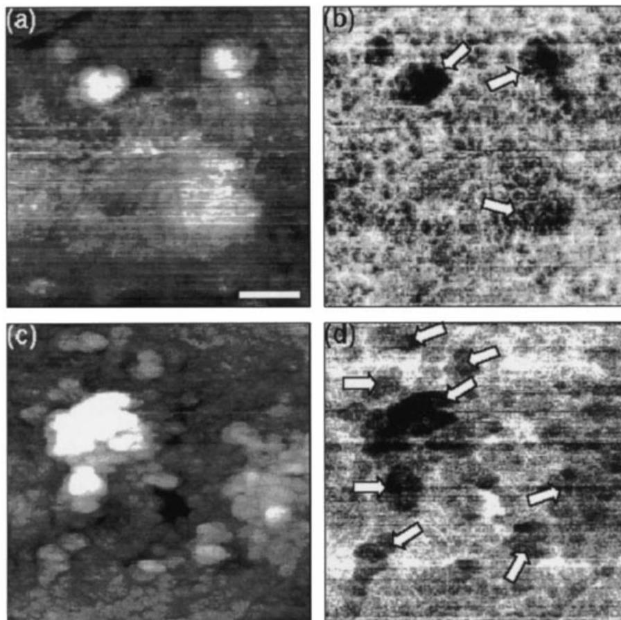
Fig. 1.  $50 \times 50 \mu\text{m}$  images of a pressed disc comprising a 50 : 50 mixture of the A and B polymorphs of cimetidine (scale bar  $10 \mu\text{m}$ ): (a) and (c) show topographical images of two different areas of the disc and (b) and (d) show the corresponding thermal conductivity images.
