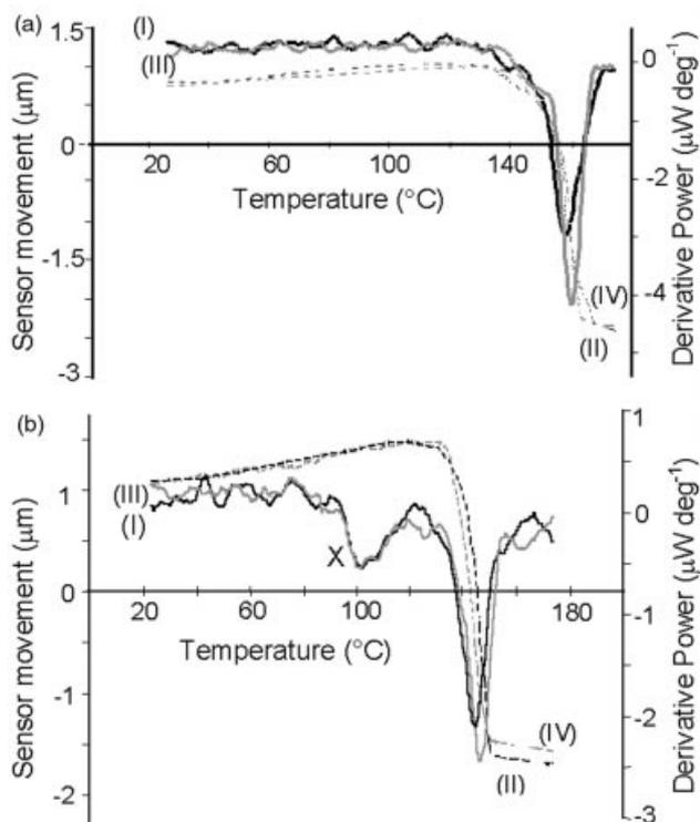
**Fig. 2.** Localized thermal analysis of a disc of pure cimetidine of (a) B and (b) A. Lines denoted (I) show the calorimetric data for a single point and dashed lines (II) show the movement of the sensor during the measurement, corresponding to thermomechanical analysis. Lines (III) and (IV) show the similar data for other points on the samples.
